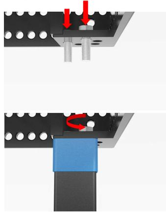
Put two fixing bolts per foot in the assembly plates.
